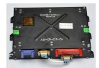
The Charge Particle Monitor (CPM), an auxillary payload in the Astrosat satellite, is designed to measure the count of charge particles at the satellite location. It is sensitive to protons above 1 MeV (Mega-electron volts). At the orbit of Astrosat (650 km), the particle rates are usually low, but, when the satellite enters
