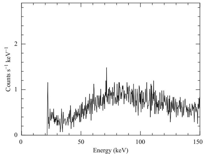
**Fig. 4.** The background spectrum from the Phoswich detector.
