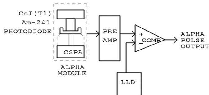
**Fig. 1.** The block diagram of Alpha-tag source with the Alpha Module and the electronics for generating Alpha pulse output for tagging the X-rays.
