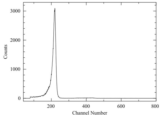
**Fig. 2.** The pulse height distribution from the Alpha-tag source. The peak corresponds to the 5.5 MeV alpha particles.
