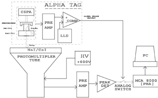
**Fig. 3.** The experimental set-up to tests the alpha tagging efficiency of the Alpha-tag source.
