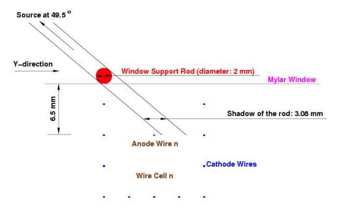
This is also for the worst case possible, with a source at  $\sim$  49.5°. The window support rod (of diameter 2 mm) casts a shadow of 3.08 mm. For this incidence,  $\sim$ 4.75 mm of the wire-cell-8 will be illuminated with the shadow of mask-pattern-1 and the shadow of 3.08 mm implies a loss of 64.72% of this effective width. The minimum loss of
