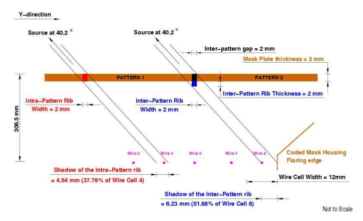
The figure illustrates the worst case possible for an incidence angle of 40.2° (with the assumed dimensions). More than 51% of wire-cell-8 is being shadowed because of inter-pattern-gap and inter-pattern-rib. The rest of wire-cell-8 and all other wire-cells will be illuminated with the shadow of mask-pattern-1 but 37.79% of wire-cell-4 will be shadowed by the intra-pattern-rib in mask-pattern-1.
