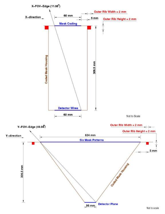
As is evident for both X and Y directions, for all possible incidences, outer ribs do not appear in the respective fields of view. Even if there is an illumination on the outer ribs, their shadows will fall on the outer side of the coded mask housing.
