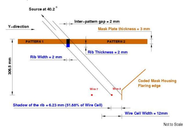
As shown in the figure, the shadow cast by the inter-pattern rib for a source at 40.2° incidence is 6.23 mm in wire-cell-8. This corresponds to a loss of 51.88% of the width of wire-cell-8; rest of the wire-cell-8 and all other wire-cells will be illuminated with the shadow of mask pattern 1. For any other relevant angle of incidence, one of the eight wires only will be affected by the shadow of one of the inter-pattern ribs (but the loss will be less than 51.88%).
